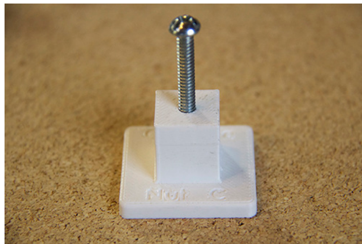
FIGURE 13 // An ABS part containing an overprinted nut. Once the part is printed, the nut is no longer visible or accessible.
