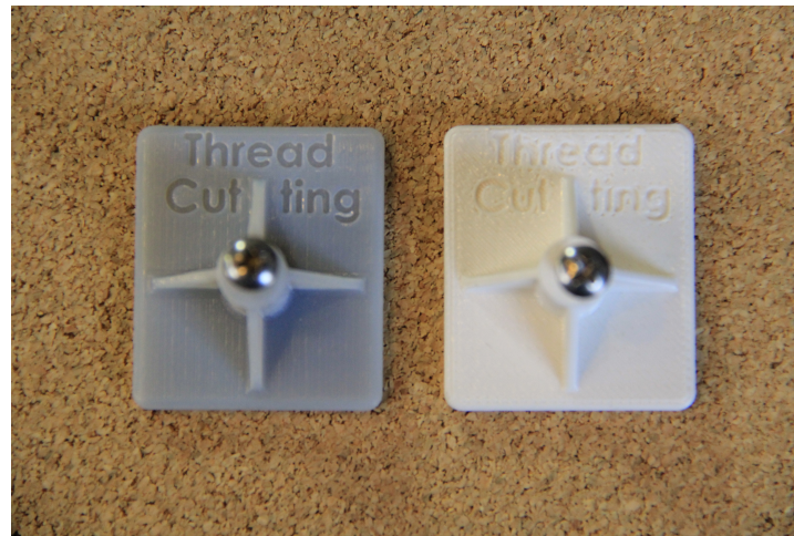
FIGURE 11 // Thread-cutting screws installed in untapped bosses in VeroGray (left) and ABS (right).
