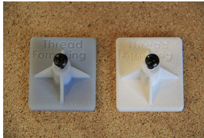
FIGURE 10 // Thread-forming screws installed in un-tapped bosses in VeroGray (left) and ABS (right).
