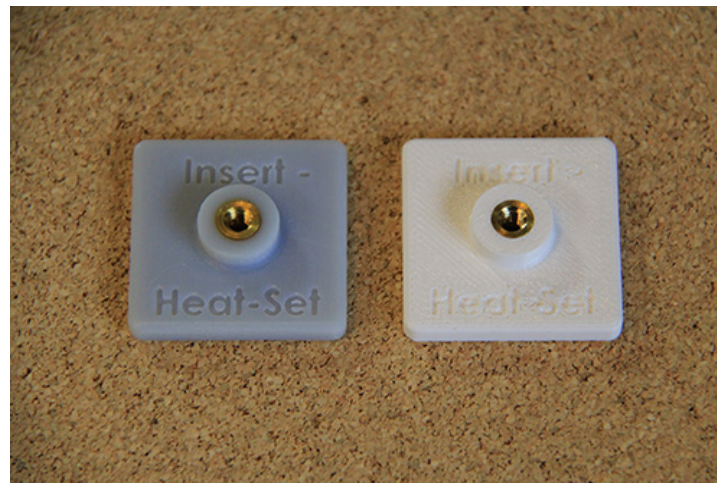
FIGURE 5 // In the PolyJet part (left), browning is visible where the hot insert burned the thermoset VeroGray, and a small fracture (not visible) formed during heated insertion. In the FDM part (right), the ABS melted and solidified, securing the insert.
