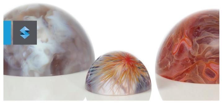
GrabCAD Voxel Print lets users control the physical characteristics of their model down to the individual voxel level, including all interior elements. This capability gives researchers and developers unparalleled control over all aspects of their 3D printed parts (research and model created by the Mediated Matter Group, Media Lab, Massachusetts Institute of Technology).
