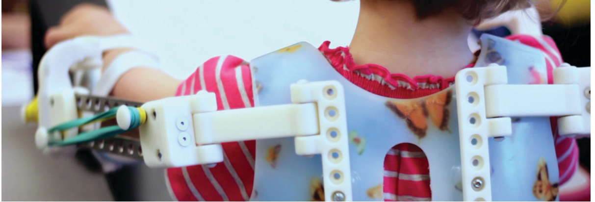
Figure 12 - Emma's smaller, customized WREX, developed using FDM technology.
