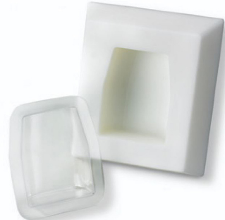
Thermoformed packaging cover and FDM mold.
