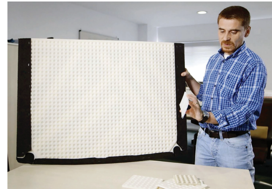
The final trunk plate produced with an FDM thermoforming tool.
