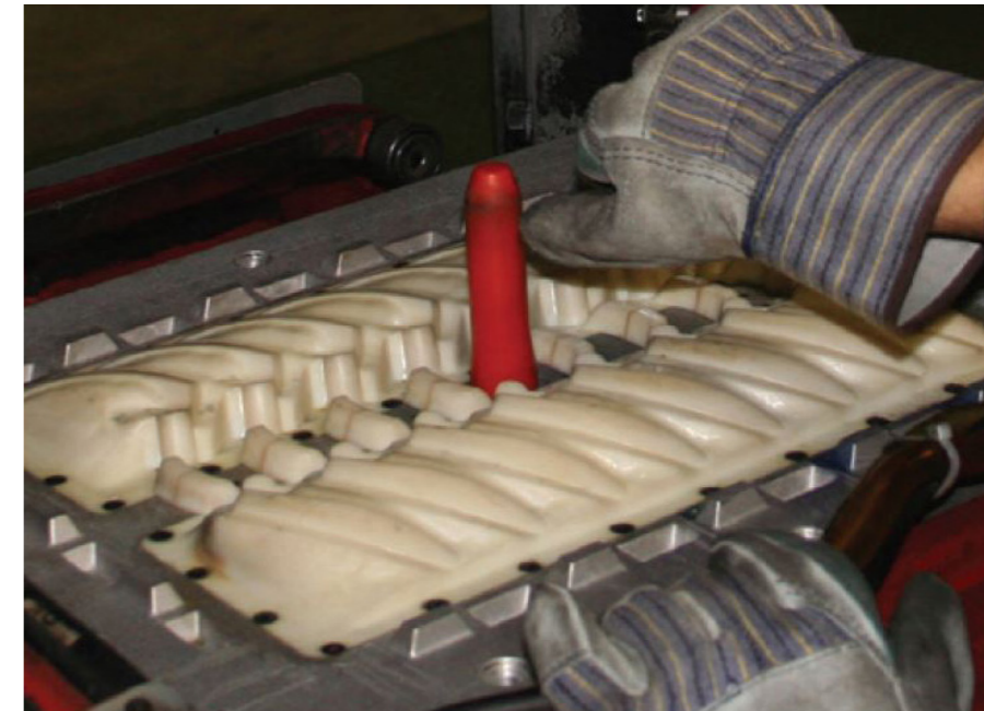
Matchplate with FDM insert in molding machine.
