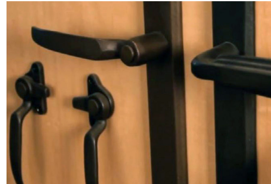
Cast door handles made using FDM patterns for sand casting.
