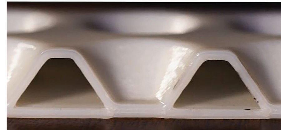
The FDM tool (top) was used to proof and then produce the dimpled design of the lightweight, twin-sheet trunk plate.
